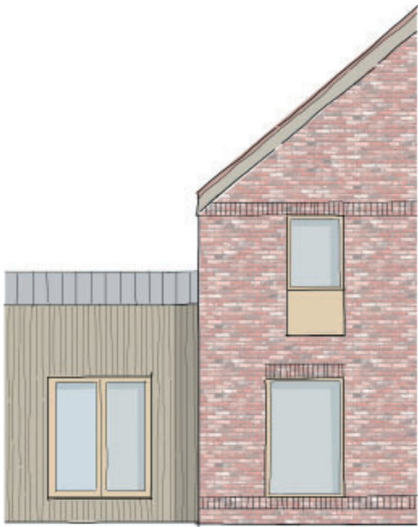
Brick: Multi Buff with Pink Hue Timber: Thermowood Weathered Wood Finish Window/Door Frames: RAL 1015
